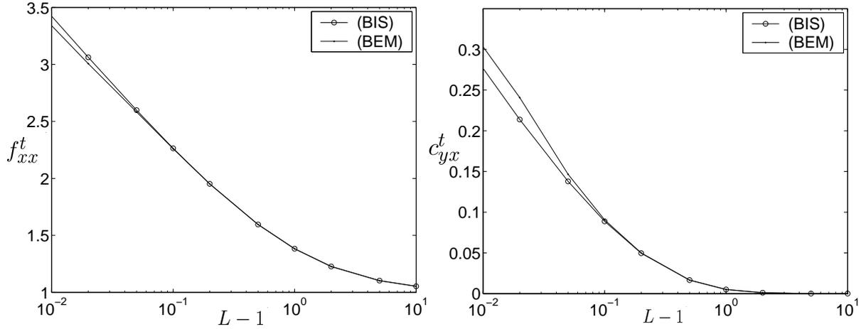
**Figure 4** Normalized drag (left) and torque (right) on a sphere translating along a wall versus the dimensionless gap  $Z - 1$  between the sphere and the wall. Our results using BEM and exact results using BIS.
