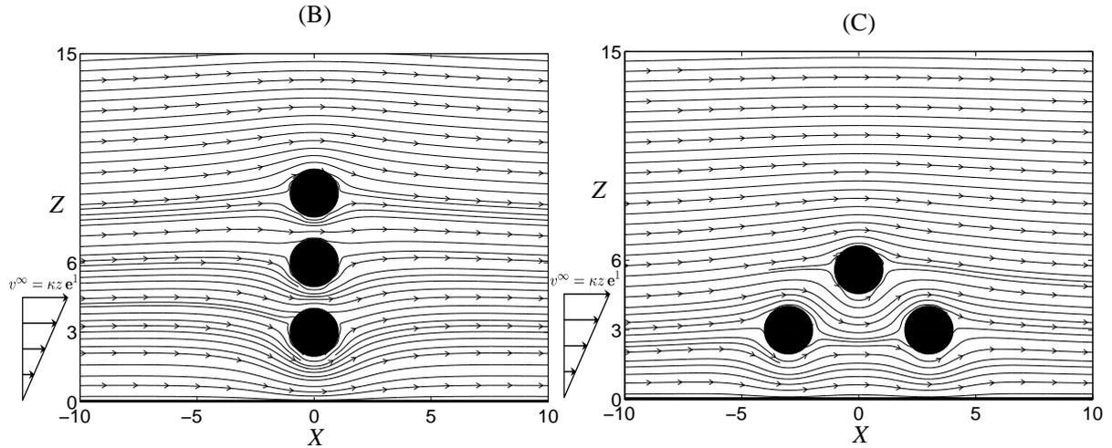
**Figure 9** Fluid trajectories around three particles fixed in a shear flow. The centers of the spheres are: (A) aligned parallel to the wall; (B) aligned normal to the wall; (C) on a the summits of a triangle. The coordinates of sphere centers are given in the text.
