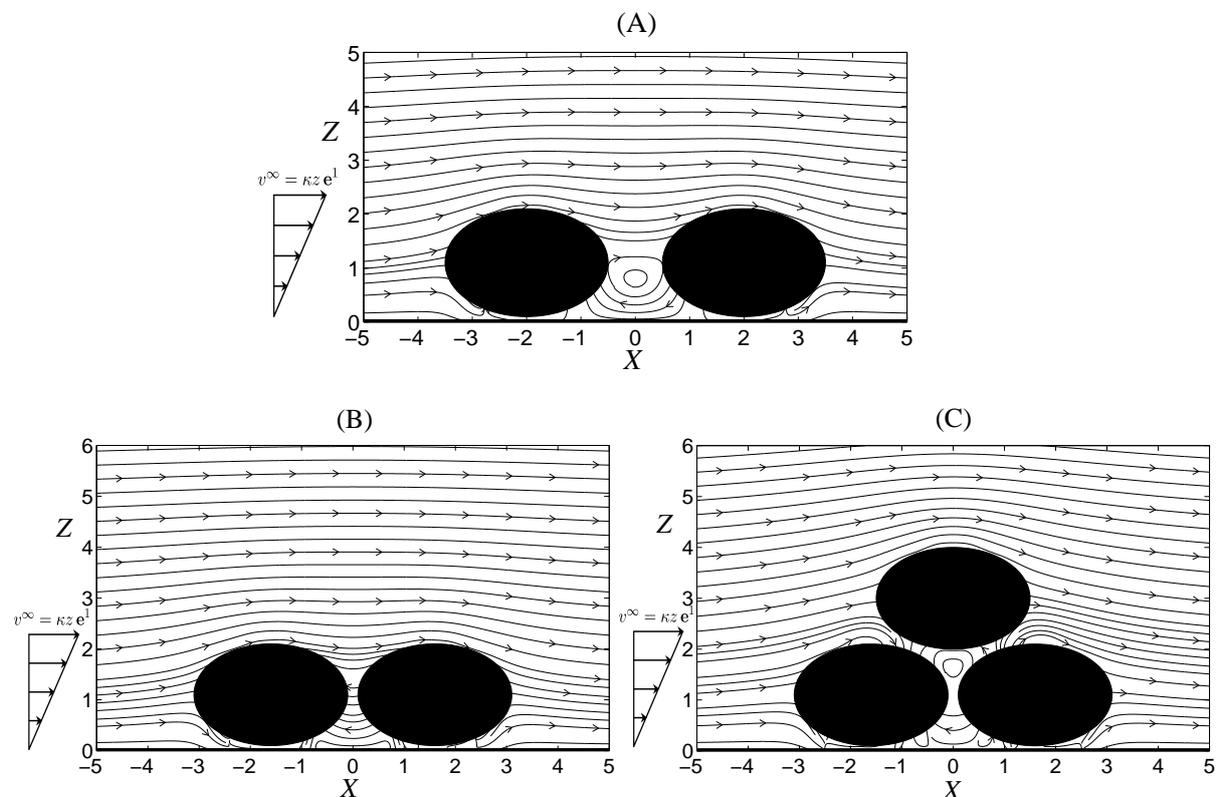
**Figure 12** Fluid trajectories around spheroidal particles fixed in a shear flow: two particles with centers at  $(-2, 0, 1.1)$  and  $(2, 0, 1.1)$  for (A);  $(-1.6, 0, 1.1)$  and  $(1.6, 0, 1.1)$  for (B); three particles centered at  $(-1.6, 0, 1.1)$ ,  $(1.6, 0, 1.1)$ ,  $(0, 0, 3)$  for (C).
