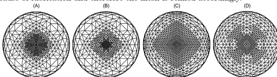
**Figure 2** Mesh refinement of a sphere in the region of high stresses, for dimensionless gaps of 0.001 (A), 0.006 (B), 0.02 (C), 0.1 (D).
