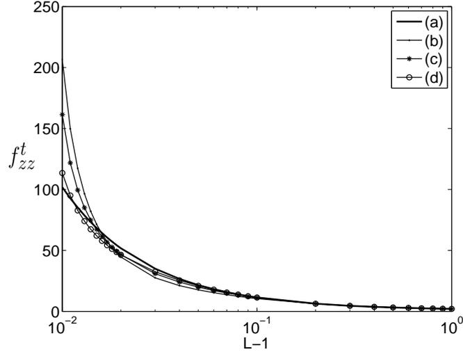
**Figure 3** Normalized drag force  $f_{zz}^t$  on a sphere settling towards a plane versus the dimensionless gap  $L - 1$ . The exact solution of [10] (a) is compared with the BEM solution using: (b) an uniform mesh at level 2; (c) an uniform mesh at level 3; (d) an adaptative mesh starting from the uniform mesh at level 2.
